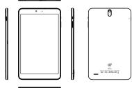
The way to turn on the tablet is to press the button, please press the power button to turn on it. Please click "power off" in the OS to turn off the tablet. Pressing the power button for several seconds by force to turn off the tablet can be used on special circumstance. What customers need to pay attention to is that frequent power-off by force may cause system files missing or crash the tablet.
